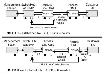
*Important:* When connecting an Access ONU with LLCF enabled to an autonegotiating device, force both sides of the configuration to the same duplex and speed. This allows the unit to immediately see link pulses and start passing data.
